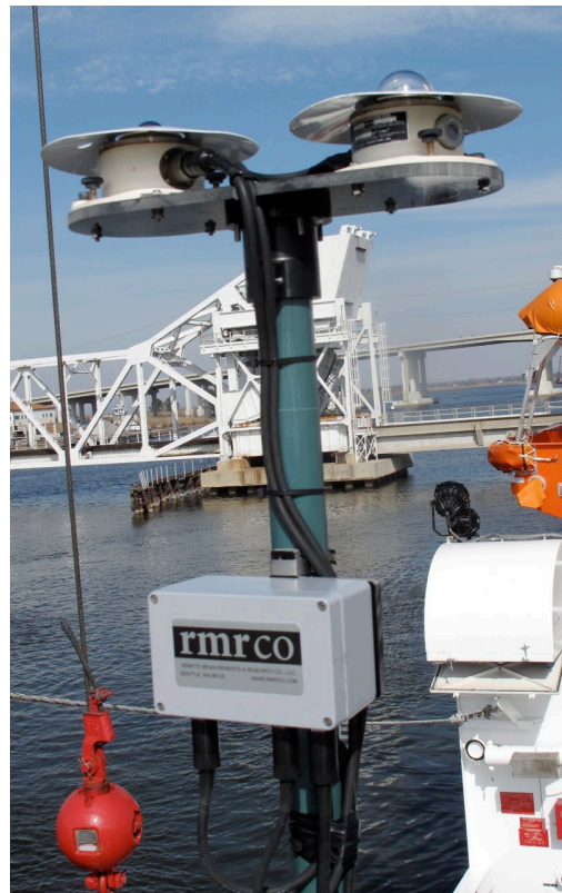
The RAD system installed on the R/V Pisces in Pascagoula MS. The mounting plates, pipe mounts, and connecting cables are provided. Installation is accomplished in minutes.
