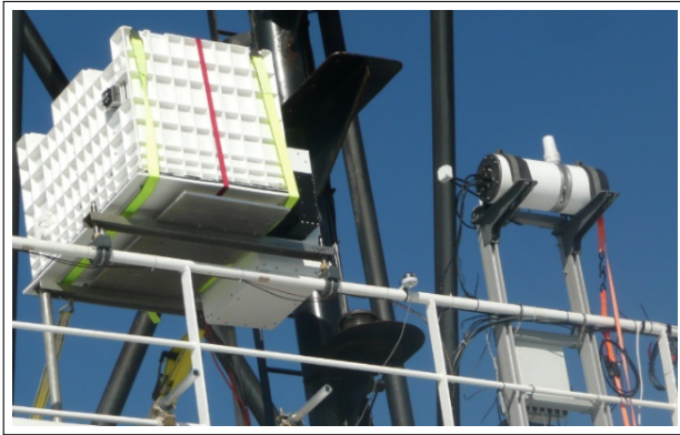
Figure 2: The M-AERI and ISAR mounted on the bridge roof forward rail staring between the two hulls.
