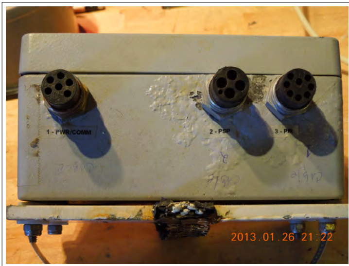
Figure 5: This enclosure has suffered severe water damage from a small nick in the connector o-ring. When the connector holes are drilled, the powder coat is broken. Normally, the receptacle o-ring prevents water getting into the break. After two years on a NOAA ship salt water penetrated under the damaged o-ring and under the powder coat finish. Extra care is taken to assure the o-rings are perfect and a sealant is used to further protect the box.
