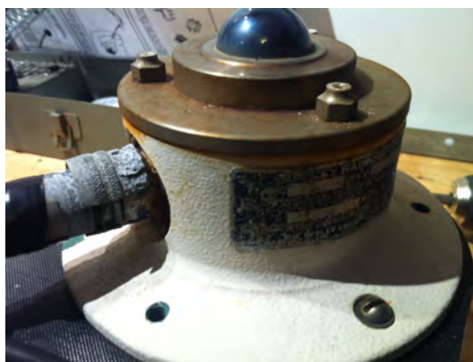
Figure 4: The PIR in this image was left unattended for several months on a tropical island in the Indian Ocean.
