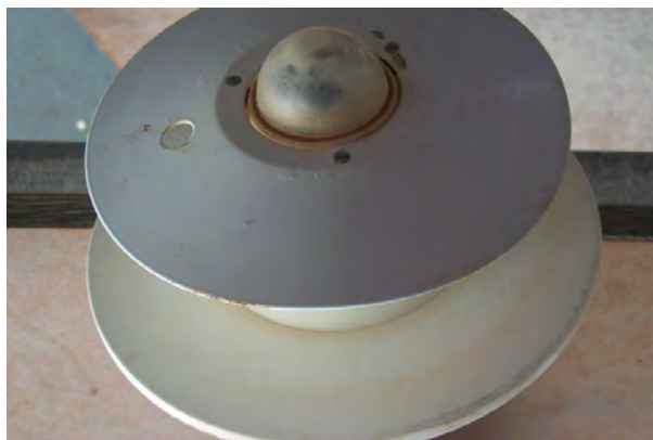
Figure 3: An accumulation of dust on a PSP from the Saharan desert. The radiometer was on a ship operating in the Carribean Sea and the deposit came across the Atlantic Ocean.
