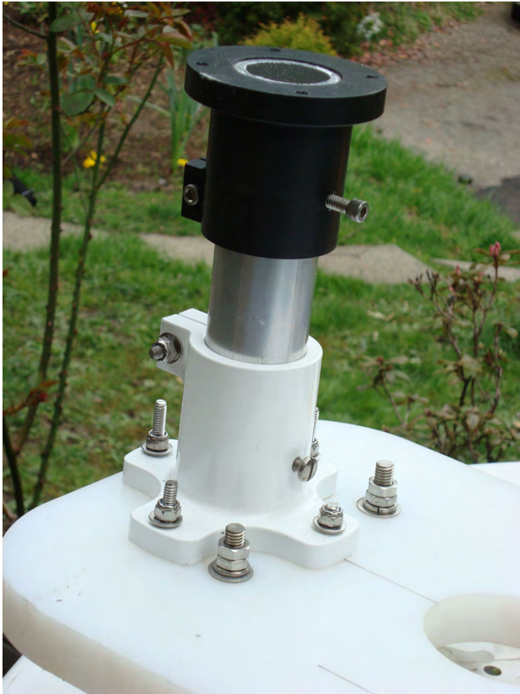
Figure 3: Two different pipe mount fittings are available for 1.5" schedule 40/80 pipe. The top pipe mount bracket is made of heavy duty plastic. It's fittings are threaded with helicoil inserts. The bottom fitting is 6061-T6 aluminum with thermoplastic powder coat.
