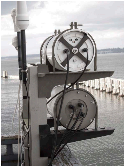
Figure 1: Left: A photograph of the ROSR and ISAR in the dual frame. Both stare down to the same spot on the lake surface. Right: Time series of the temperatures measured by the two instruments. Time begins on 5/16.
